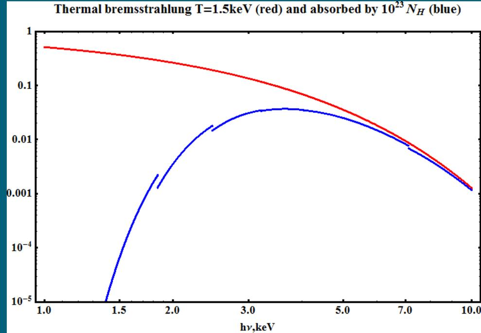
At  $N_H=10^{23}\text{cm}^{-2}$ , peak energy reaching the detector is  $\geq 4\text{keV}$
